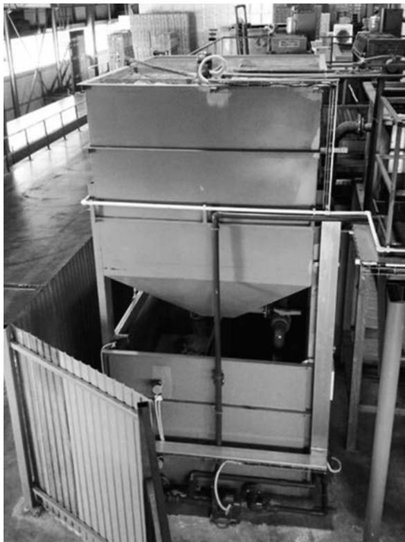
**Fig. 4.5.** Photo of industrial sample of flotodecanter
